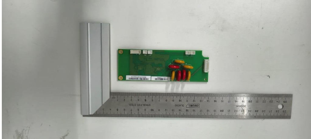
Photo 59: View of the Inlet_board supplied by three phases
