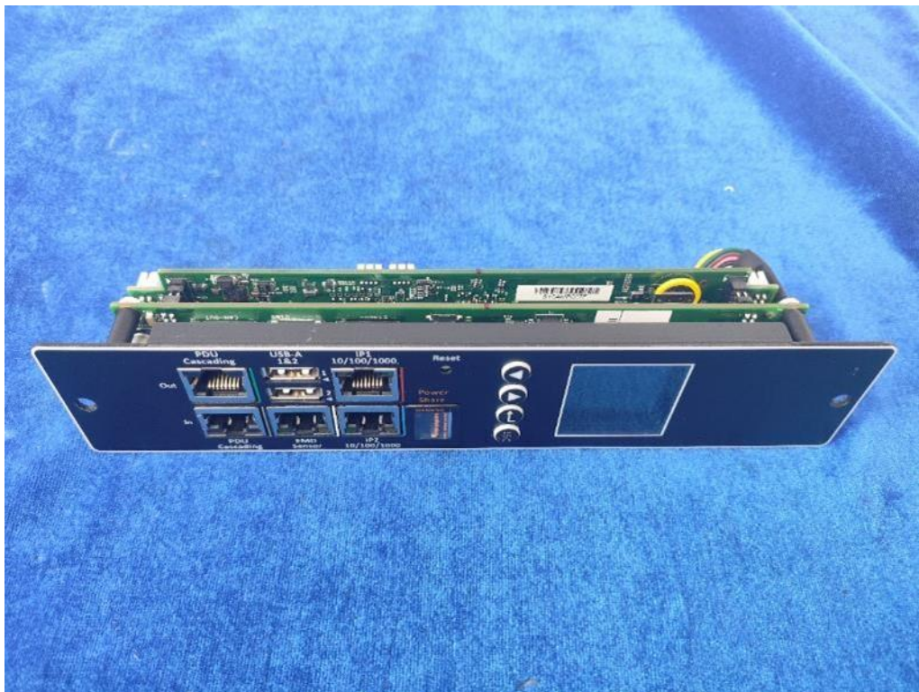
Photo 38: View of the terminal, control &amp; display module of SPIM, SPOM, SPOS, SPOX series
